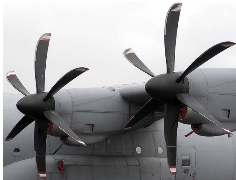
Figure 4.10: A C-130 Hercules with its propellers feathered
