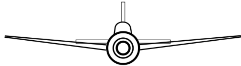
Figure 0.2: Wing dihedral, the upward angle of the wings, illustrated (thanks to Wikimedia Commons user Steelpillow for the image)
