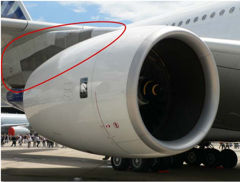
Figure 0.4: An Airbus A380's engine pylon (thanks to Wikimedia Commons user David.Monniaux for the photo)
