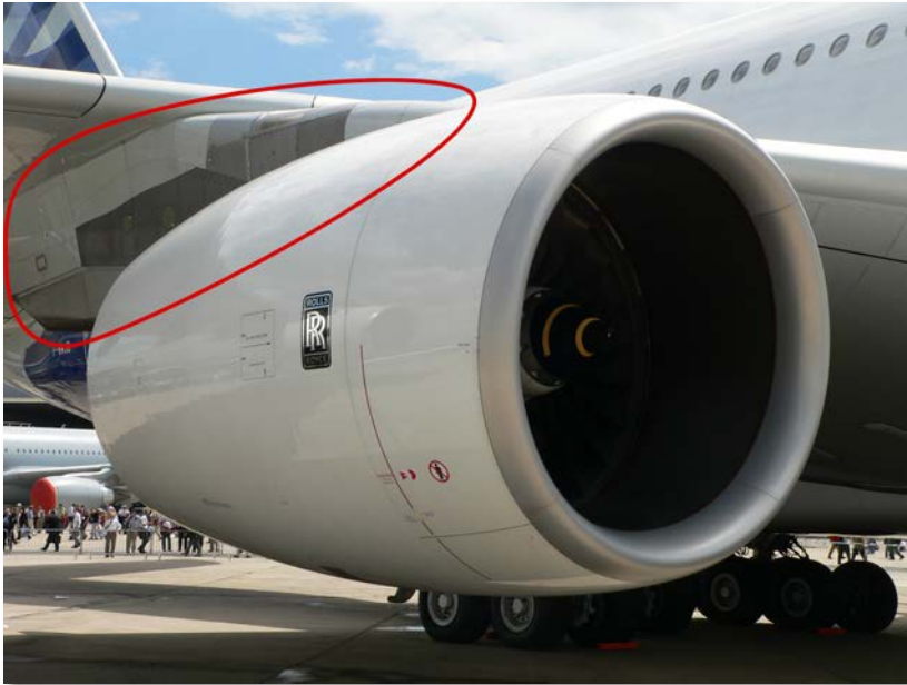
Figure 3.46: An Airbus A380's engine pylon (thanks to Wikimedia Commons user David.Monniaux for the photo)
