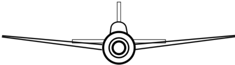
Figure 3.31: Wing dihedral, the upward angle of the wings, illustrated (thanks to Wikimedia Commons user Steelpillow for the image)
